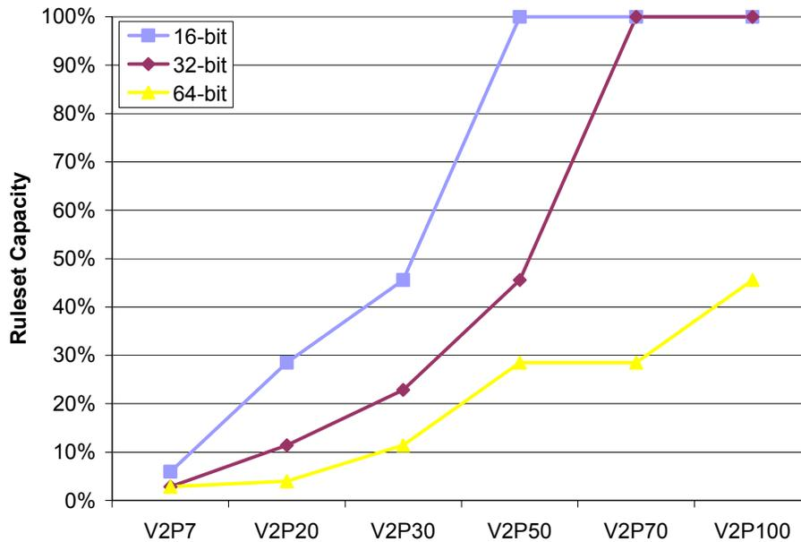
Figure 7: Rule set capacity of different FPGA devices
