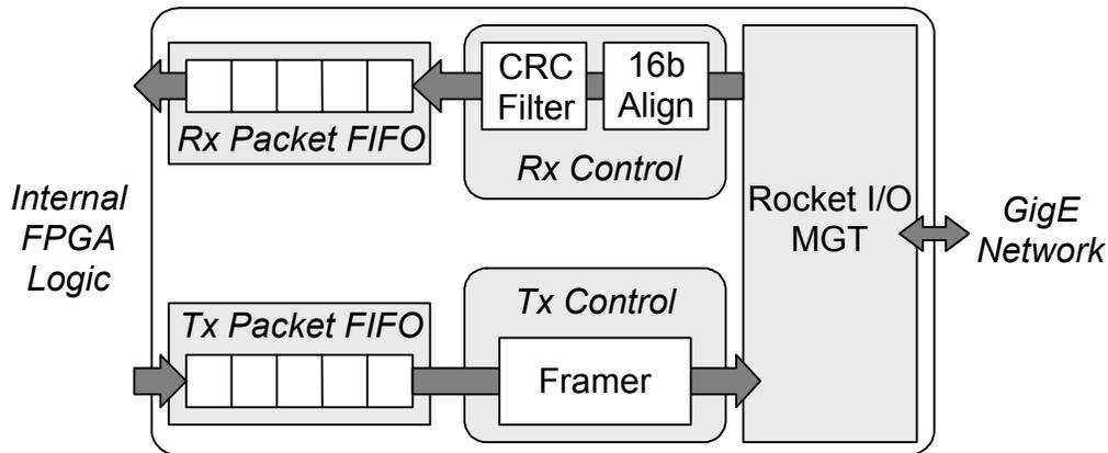
Figure 1: Gigabit Ethernet network interface module
