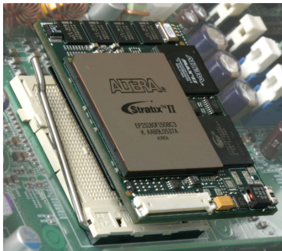
Figure 7: The XtremeData 1000 FPGA accelerator features an Altera FPGA that plugs into a standard AMD Opteron socket and communicates with the host using HyperTransport. 7
