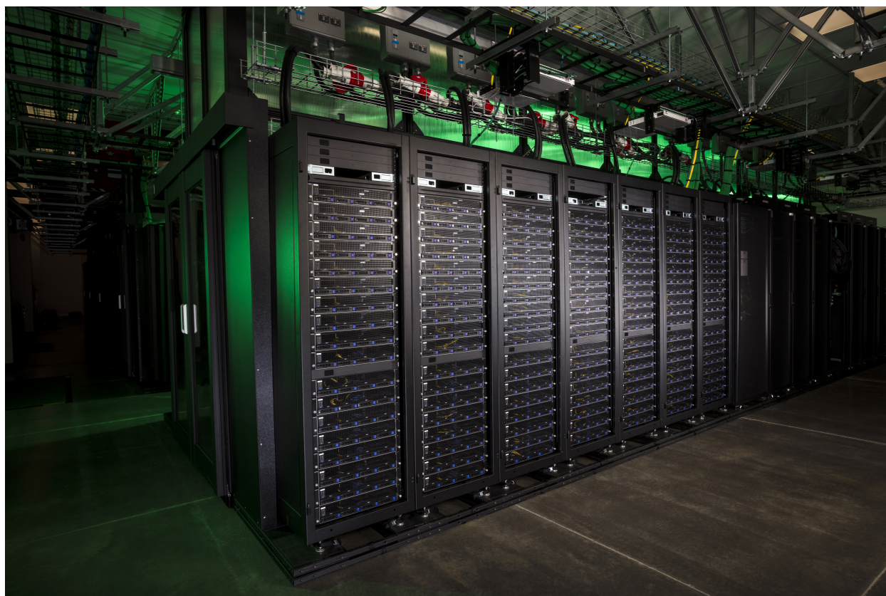
Figure 3-4. Compute nodes are stored in seven racks, with networking at the top
